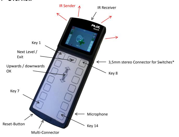
\* Pilot touch automatically detects whether single switch (mono plug) or a dual switch (stereo plug) is connected. See the icons below that will appear in the display while the connector is in use.
