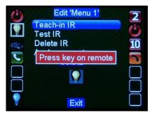
Position the remote control again in front of the PILOT touch as shown and press the desired key you want to copy. If there is a signal recognized you can see a blinking icon in the PILOT touch display.
